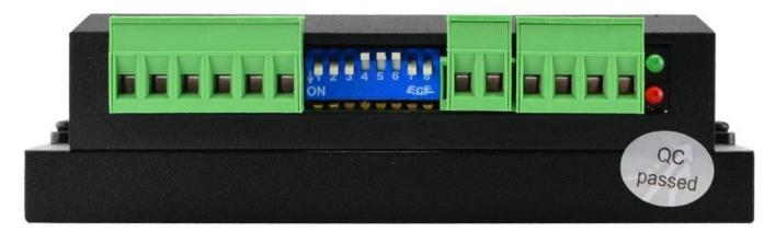
We also see here that the microstep driver is set for SW5=Off, SW6=Off, SW7=On, and SW8=On. We can check the table that is printed on the M542 faceplate and find that these setting produce a microstep configuration for 1600 steps per revolution.
