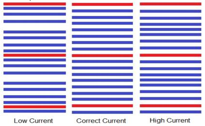
This graphic shows a position representation for a motor with 8 microsteps. The odd spaced shows that a low current for the coils will not be strong enough to correctly pull the (blue) shaft position between the (red) poles. Having too high of current applied will cause an unwanted result of motor shaft position as well. A properly tuned motor and microstep driver should be able to work together to attain the consistent spacing between magnetic poles.
