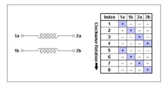
If the steps are continuously being commanded, then the stepper movement appears to be a smooth, continuous rotation.
